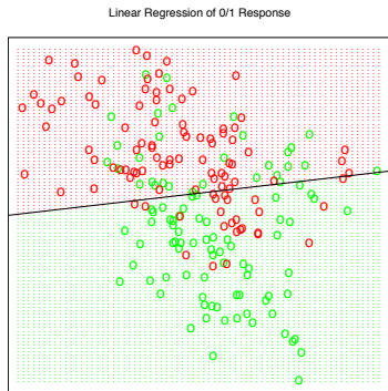
Figure 2.1: A classification example in two dimensions. The classes are coded as a binary variable— GREEN = 0, RED = 1—and then fit by linear regression. The line is the decision boundary defined by x^T \hat{\beta} = 0.5 .
